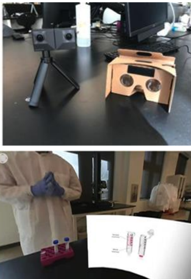
Figure 6. The Insta360 EVO VR camera in 180° 3D mode and the Google Cardboard headset used for VR videos of the laboratory component of a Biomolecular Engineering course. (Reproduced under the terms of CC BY-NC 4.0)
